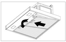
3. Reinstall the aluminium filter in its slot after flushing by following the above steps in reverse.
